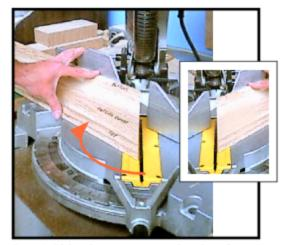
Cut 1 Side then Reverse the Cut for the 2nd side. (Outside Corner Shown)
