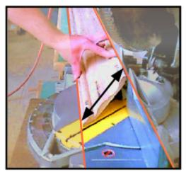
Mark a line on the Fence and Table Use this Line to **Keep the Same Angle**
